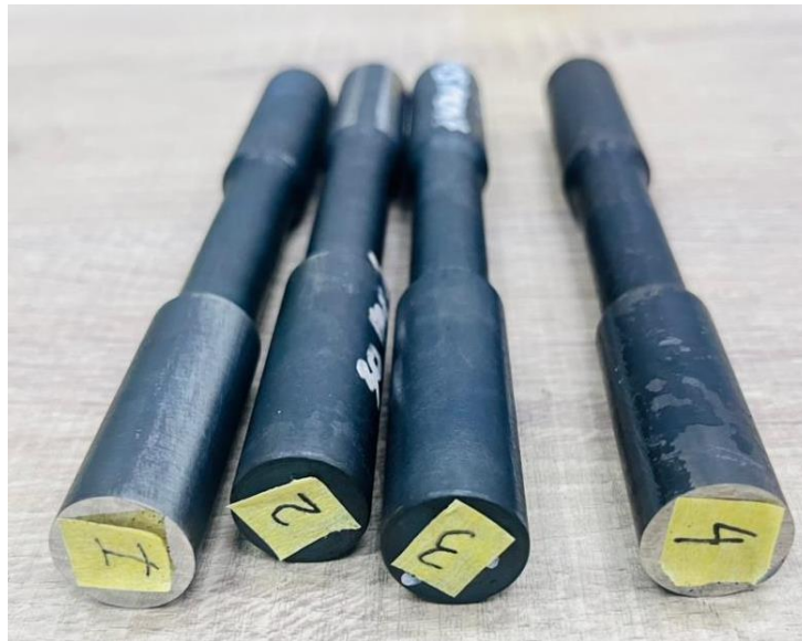
Gambar 3.9 Material S45C setelah diproses perlakuan panas ( heat treatment )
